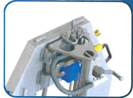
Cutter feed motion is controlled by a feed screw and crank handle on top of the tool.
